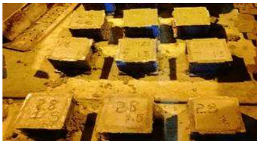
Fig. 7: Casted Cube Specimens
