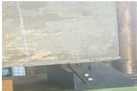
Fig. 13: Observed first crack on the conventional slab specimen at load 105 KN
