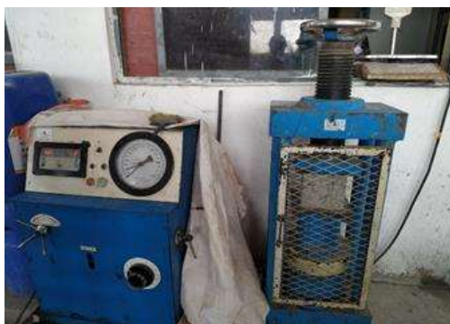
Fig. 11: Compression Testing of Cube
