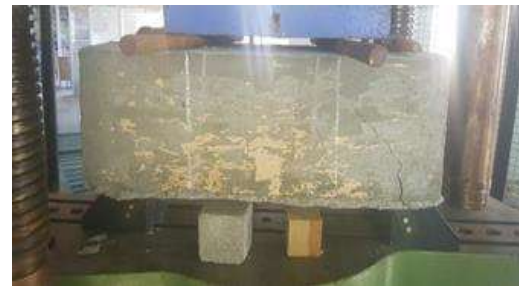
Fig. 12: Two Point Load Testing of Slab Specimen
